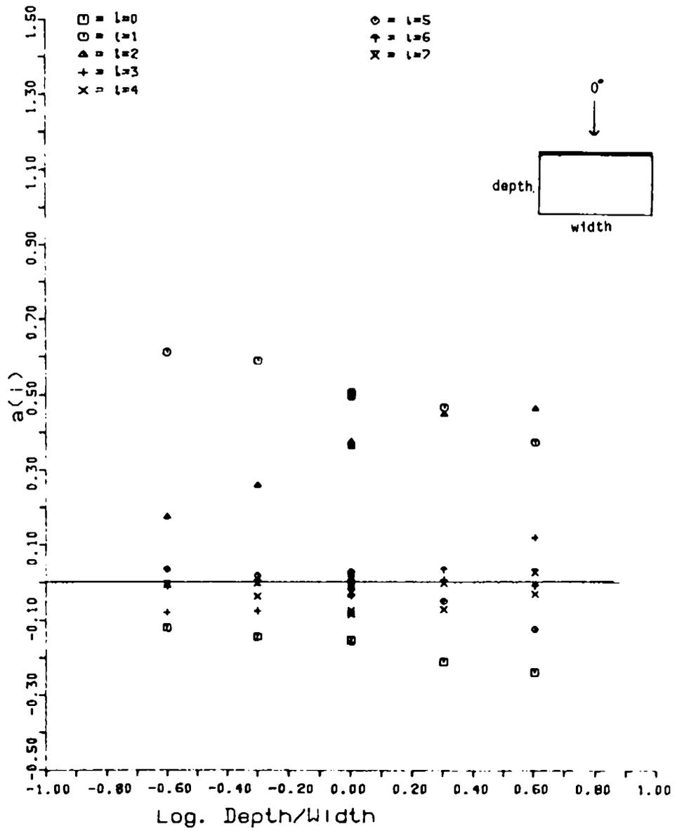
Fig.(7.2) Coefficients  $a(i)$  for roof level pressure coefficients.
