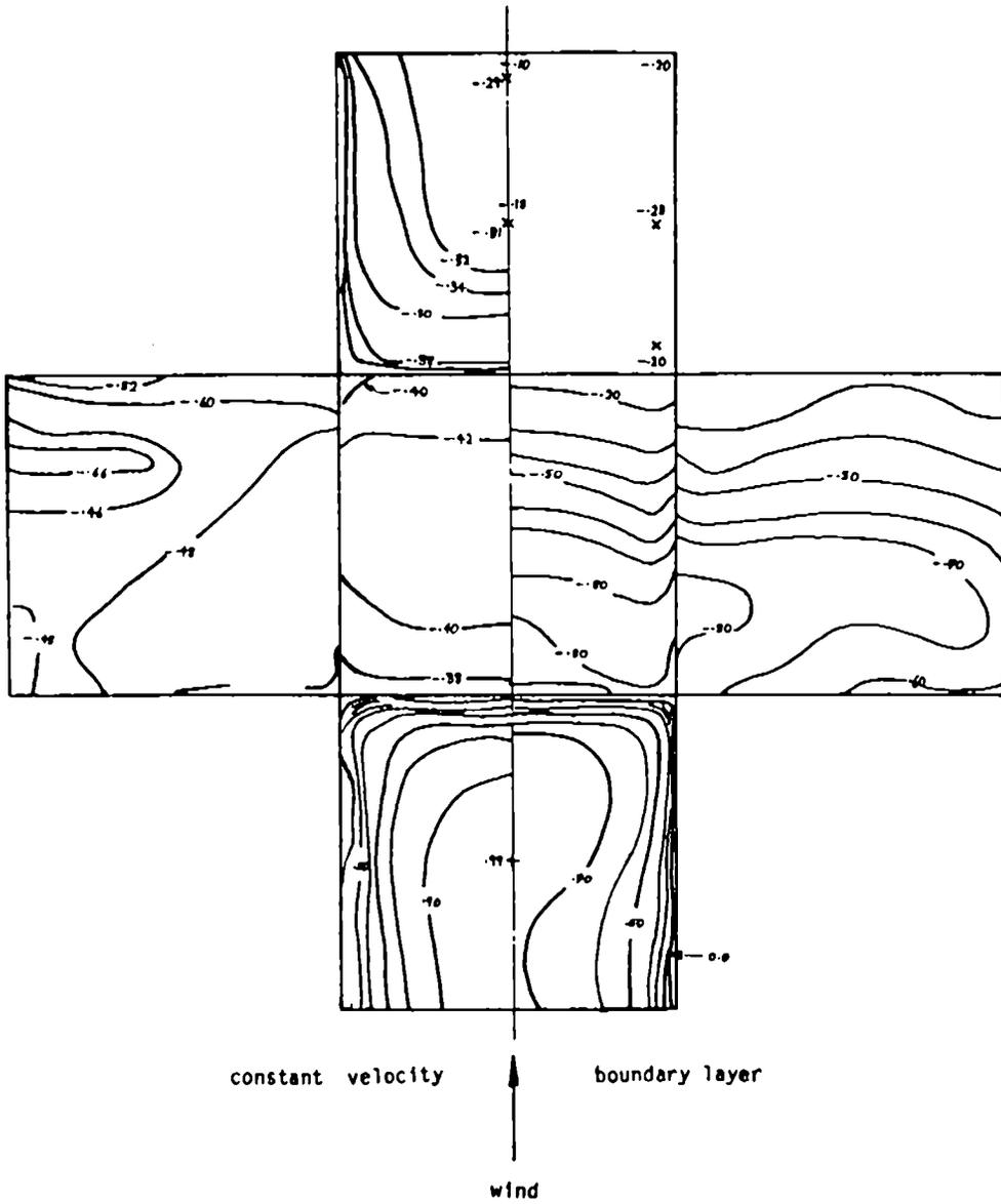
Fig.(3.10) Comparison of pressure coefficients on a cube for constant velocity and boundary layer flow. (after Hamilton<sup>25</sup>)
