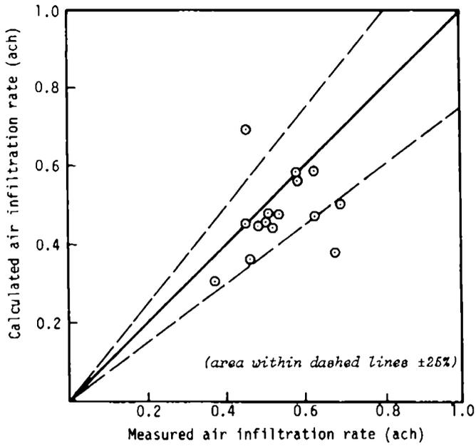
Fig.(1.5) Measured vs. calculated infiltration rates for the Runcorn House, using NRC pressure coefficients.
