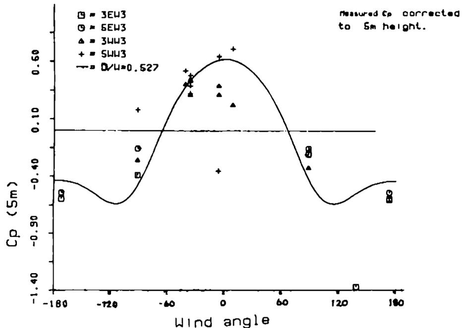
Fig.(7.12b) Measured and calculated pressure coefficients plotted against wind angle for the Aylesbury test house.
