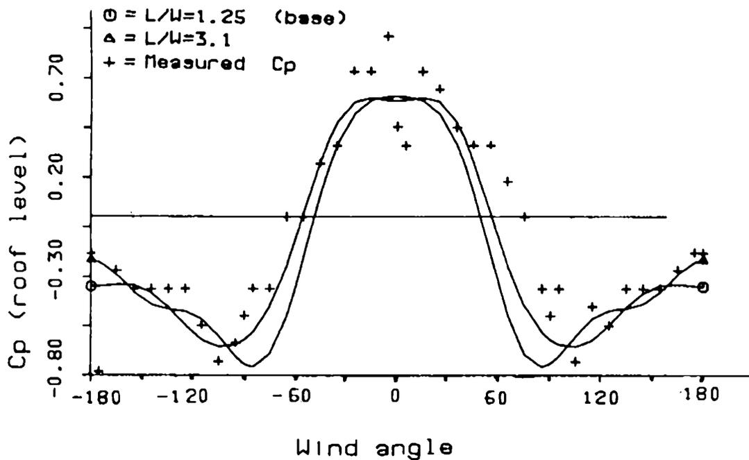
Fig.(7.8b) Measured and calculated pressure coefficients plotted against wind angle for position 18 (end wall).
