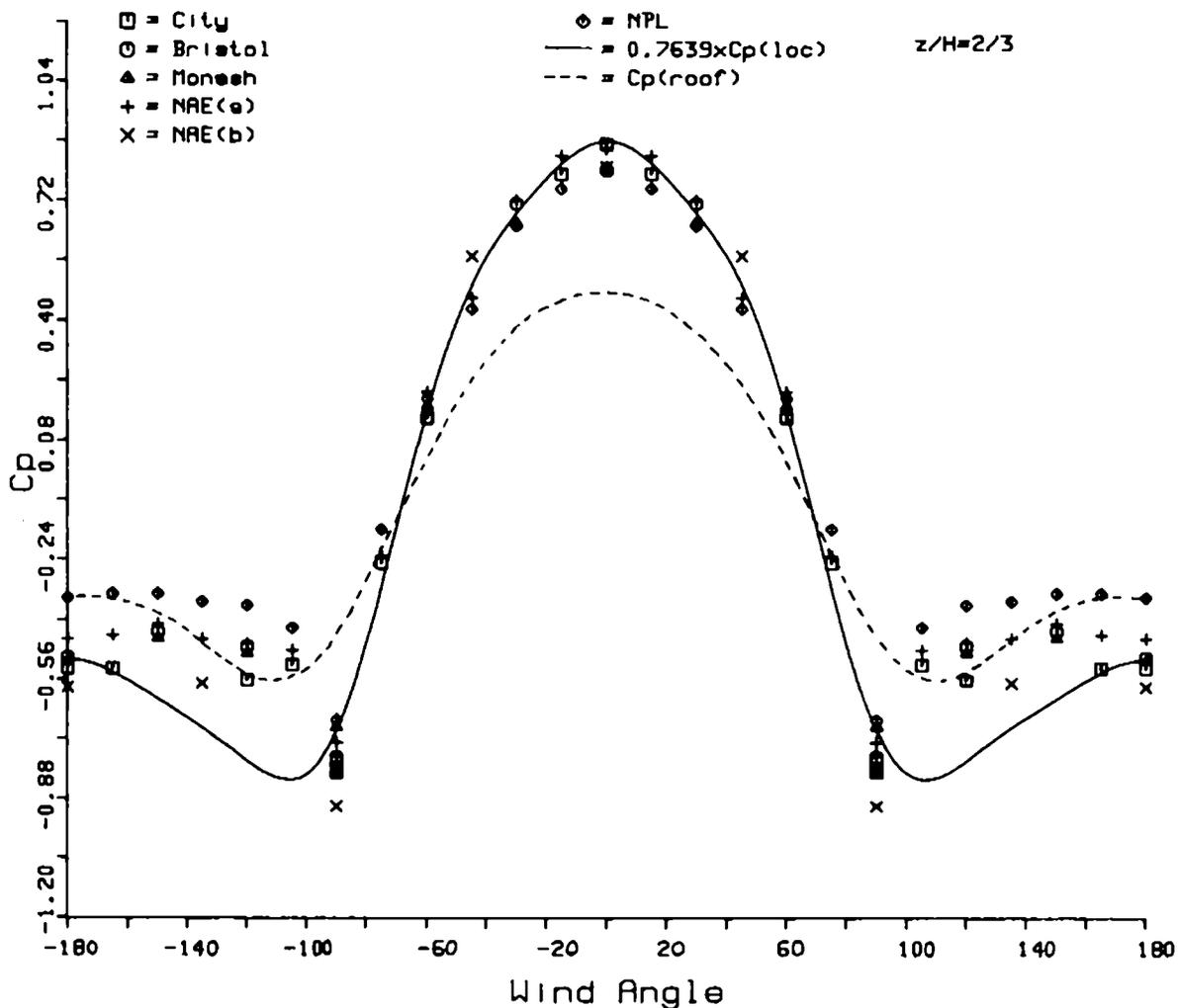
Fig.(7.13) Measured and calculated pressure coefficients plotted against wind angle for the CAARC Standard Tall Building Model.
