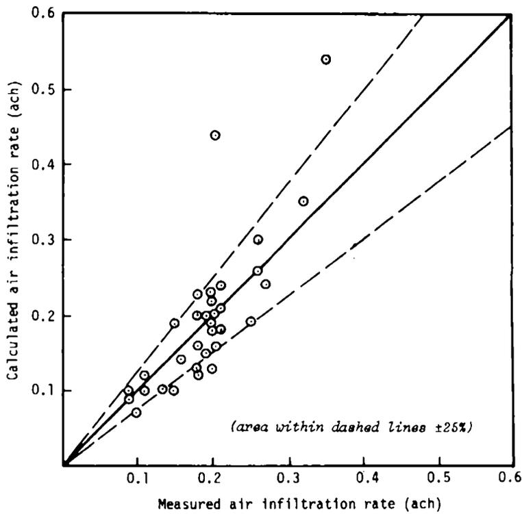
Fig.(1.3) Calculated vs.measured infiltration for the HUDAC Mk XI house using CP3 pressure coefficients. ('upgraded house')
