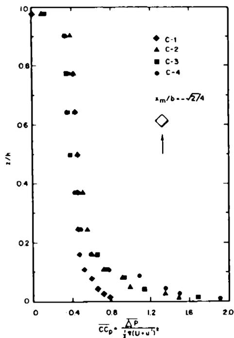
Vertical distribution of corrected mean pressure coefficient ( $n=1$ ) on windward face of building in orientation I.
