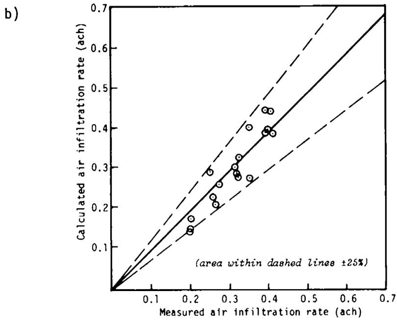
Fig.(1.1a) Case by case comparison of observed and calculated infiltration rates for the Maugwil House.
