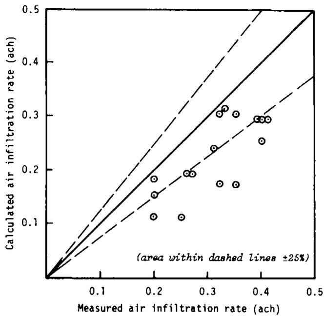
Fig.(1.6) Measured vs. calculated infiltration rates for the Mougwil House, using NRC pressure coefficients.
