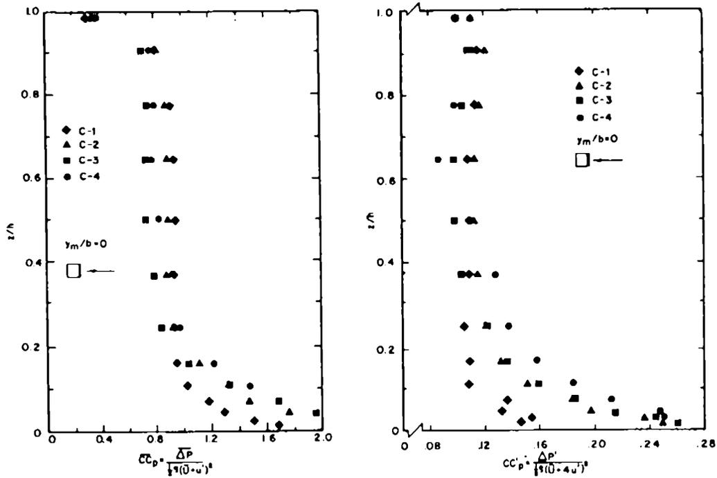
Vertical distribution of corrected mean pressure coefficient ( $n=1$ ) on windward face of building in orientation II.
