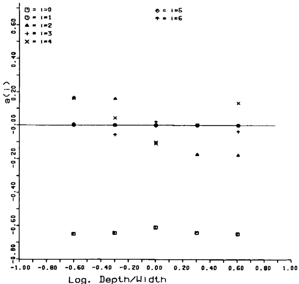
Fig.(7.6) Coefficients  $a(i)$  from eqn. 7.1 for the mean  $C_p$  of a flat roof. (same for both roof level and local reference winds)
