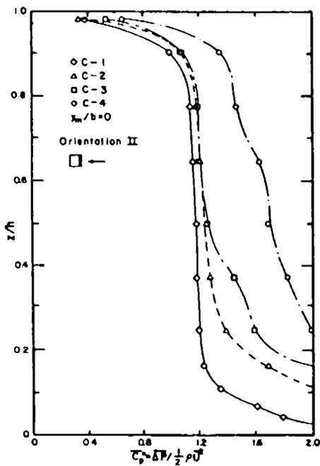
Vertical distribution of local mean pressure coefficient on windward face of building in orientation II.
