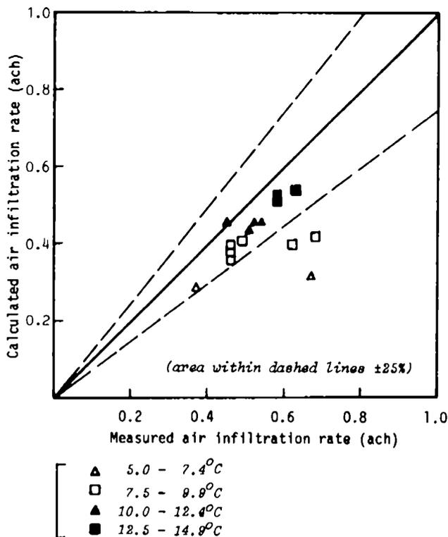
Fig.(1.4) Measured vs. calculated infiltration rates for the Runcorn House. (stack effect only)
