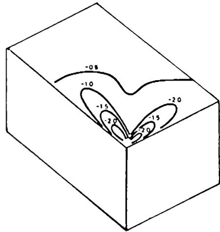
Fig.(3.7) Pressure distribution over the roof.
