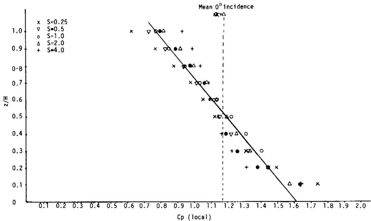
Fig.(7.10) Local pressure coefficients for zero wind angle and various S plotted against z/H.
