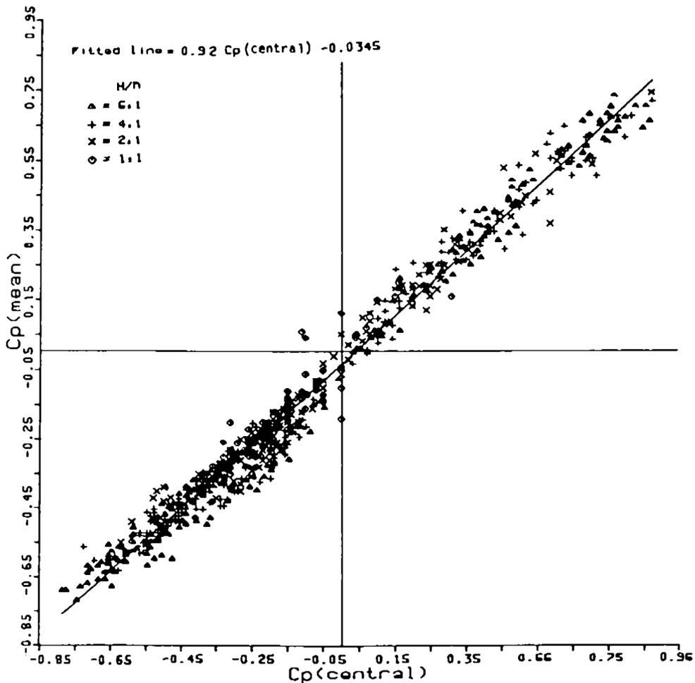
Fig.(7.9) Plot of mean Cp against centre line Cp for various z/H, H/h and wind angle for face A.(see Fig.(7.4)) (data from Bowen<sup>67</sup>)
