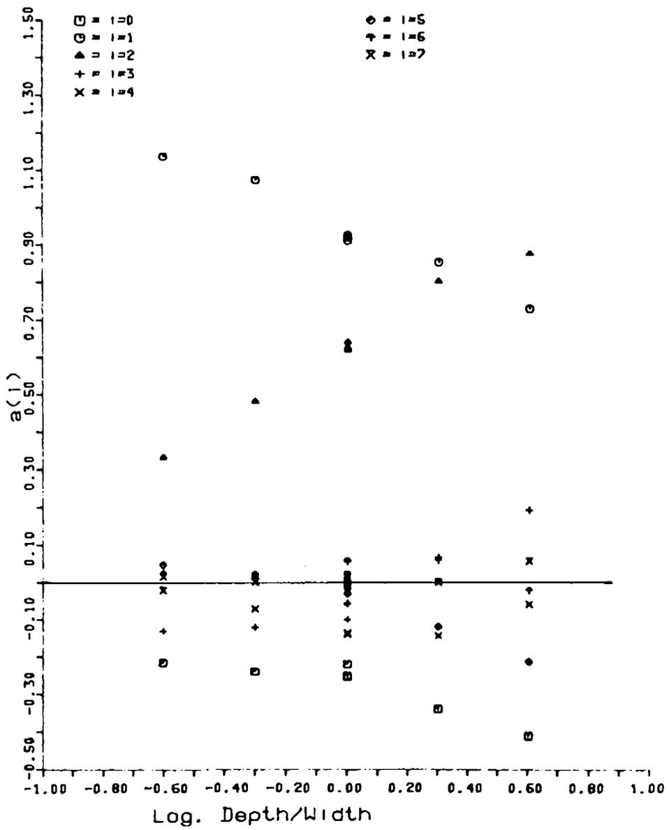
Fig.(7.3) Coefficients  $a(i)$  for local pressure coefficients.
