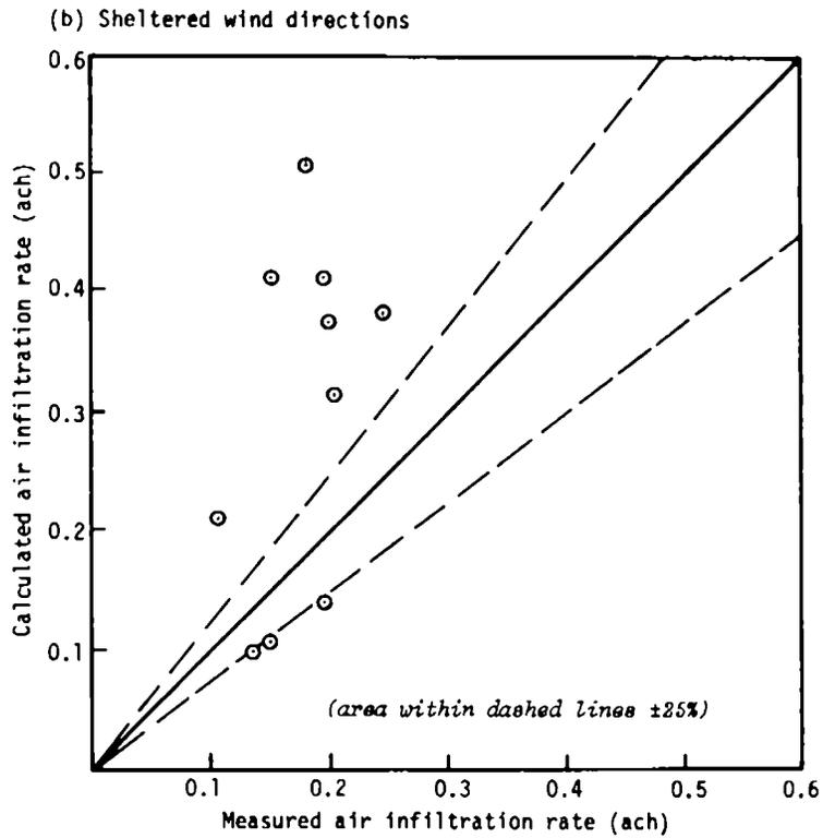
Fig.(1.2) Measured vs. calculated infiltration rates for the HUDAC Mk XI House.(using CP3 pressure coefficients)
