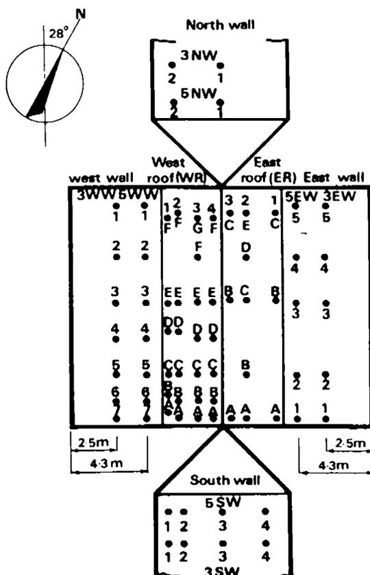
Fig.(7.11) Aylesbury Test House - location of pressure taps
