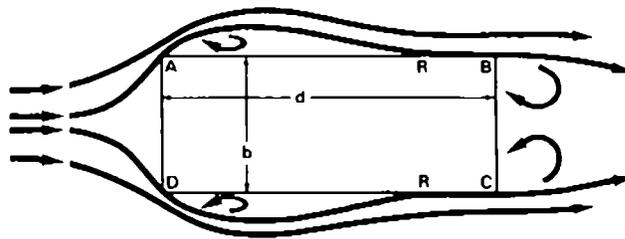
Fig.(3.3) Illustration of flow reattachment.
