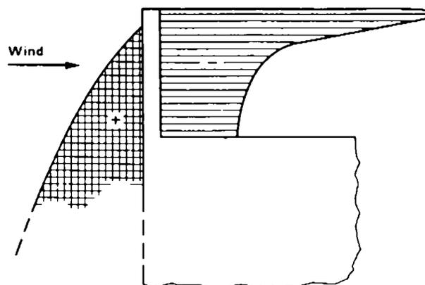
Fig.(3.9) Pressure distribution on a roof parapet (section).
