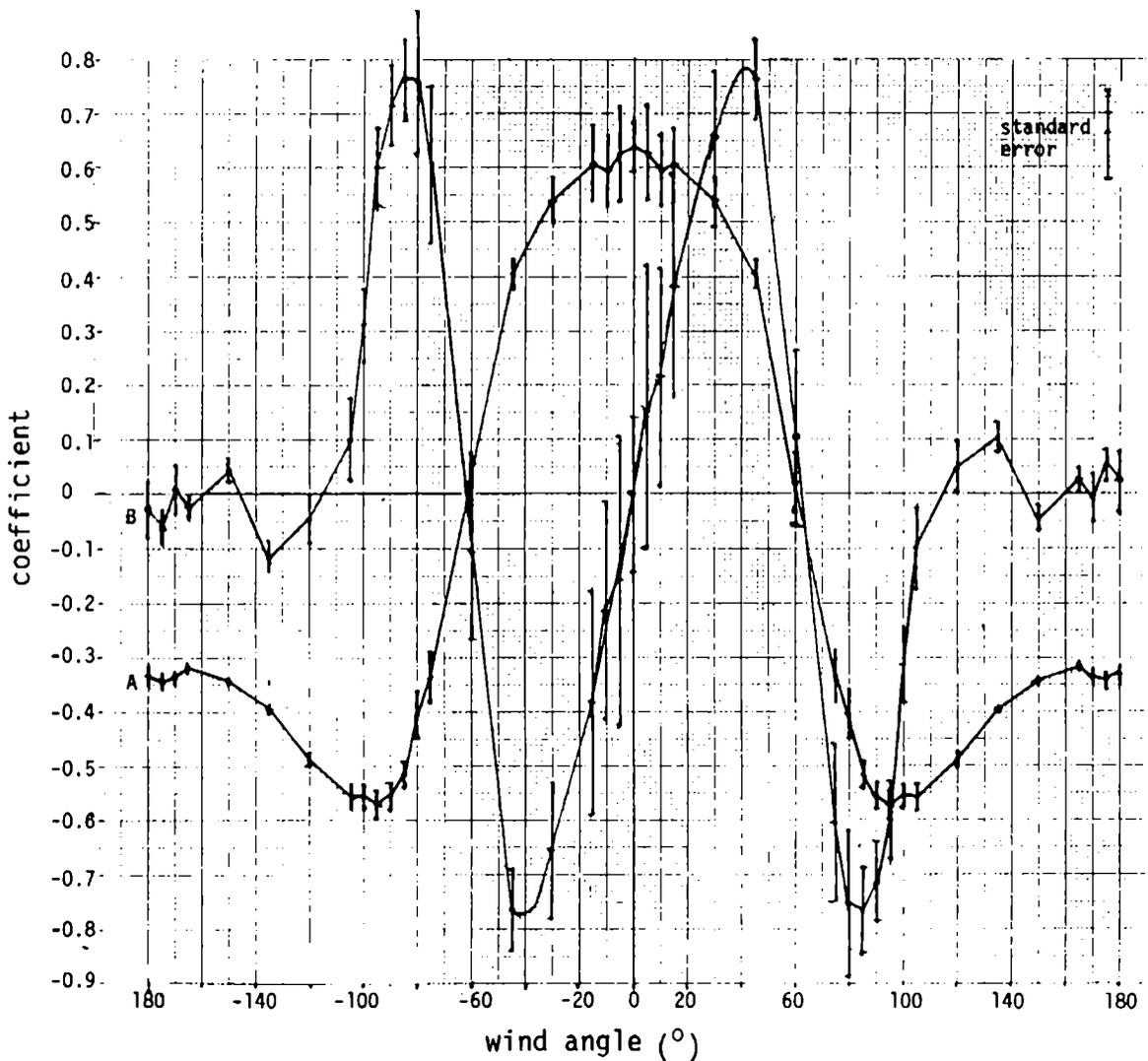
Fig.(7.5) Fourier analysis of the horizontal pressure distribution across a facade with wind angle. (see eqn. 7.2) (data from Bowen<sup>67</sup>)
