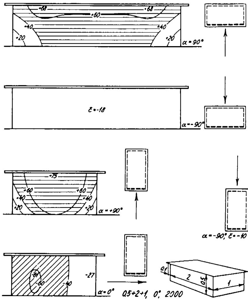
Fig.(3.8) Pressure distribution on a model building with overhanging eaves. (Jensen and Frank<sup>17</sup>)
