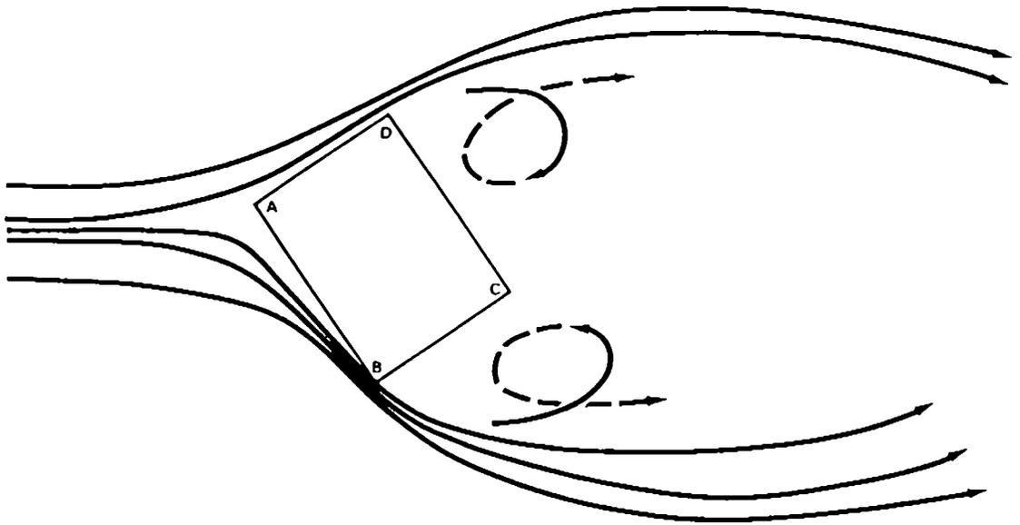
Fig.(3.4) Plan view of flow around a rectangular building with oblique wind incidence.
