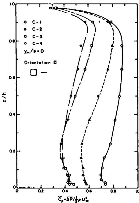
Vertical distribution of mean pressure coefficient along centerline of windward face of building for orientation II.
