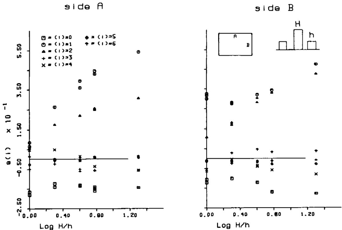
Fig.(7.4) Coefficients  $a(i)$  as a function of shelter ( $H/h$ ).
