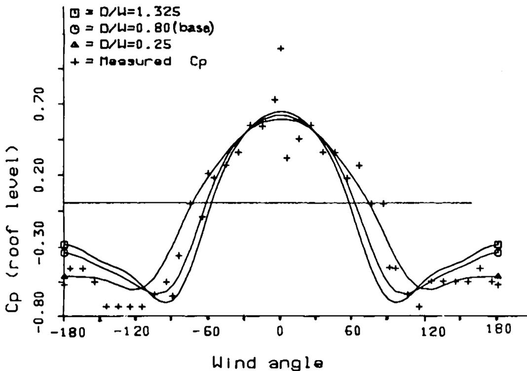
Fig.(7.8a) Measured and calculated pressure coefficients plotted against wind angle for position 6 (side wall).
