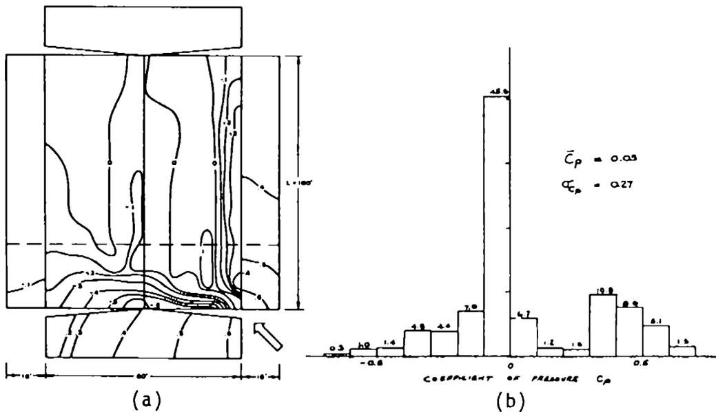
Fig.(2.1) a) Pressure distribution on a low rise building for a wind angle of 45 degrees.
