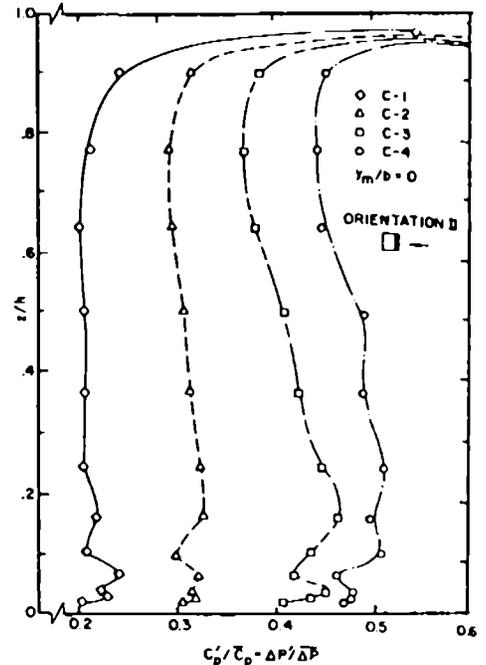
Vertical distribution of fluctuating pressure intensity along centerline of windward face of building for orientation II.
