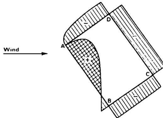
Fig.(3.5) Pressure distribution on the walls.
